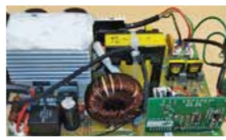
SMPS Battery chargers
